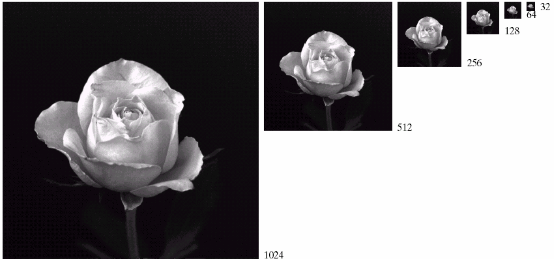
FIGURE 2.19 A 1024 \times 1024 , 8-bit image subsampled down to size 32 \times 32 pixels. The number of allowable gray levels was kept at 256.
